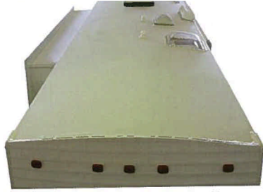
3/8" crowned truss, walk on roof decking.
